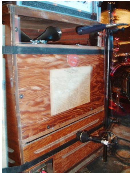
Cobalt Co4 instrument mic on top of Leslie (rotating HF horn); N/D468 on LF portion of Leslie cabinet
