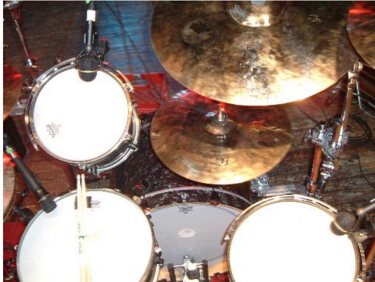
(l-r): N/D478 on snare; N/D468 on rack tom; RE200(s) on cymbals (not pictured); N/D468 on floor tom; N/D868 on kick drum (not pictured)
