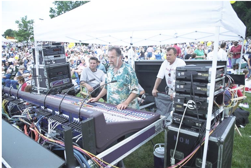
(l-r) Brent Alwin (Independent Engineer), Terry Tilley (MN Orchestra engineer), Greg Ecklund (President/Engineer Urban Communications) with Midas Legend 3000 and Klark Teknik Helix EQ
