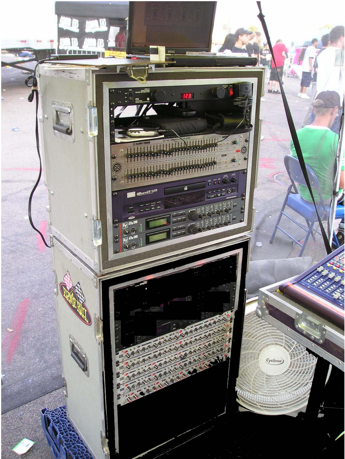
Klark Teknik DN360 graphic equalizer, EV Dx38 DSPs, Klark Teknik DN500 Plus dynamic processors
