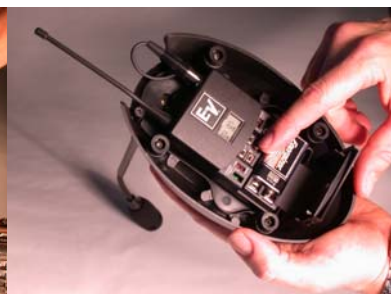
Programmability & changing batteries are facilitated without removal of transmitter from the satellite base
